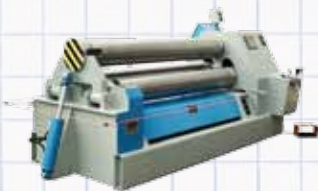
101-10-8 (1/2" x 8') hydraulic pinch pyramid plate bending machine.
