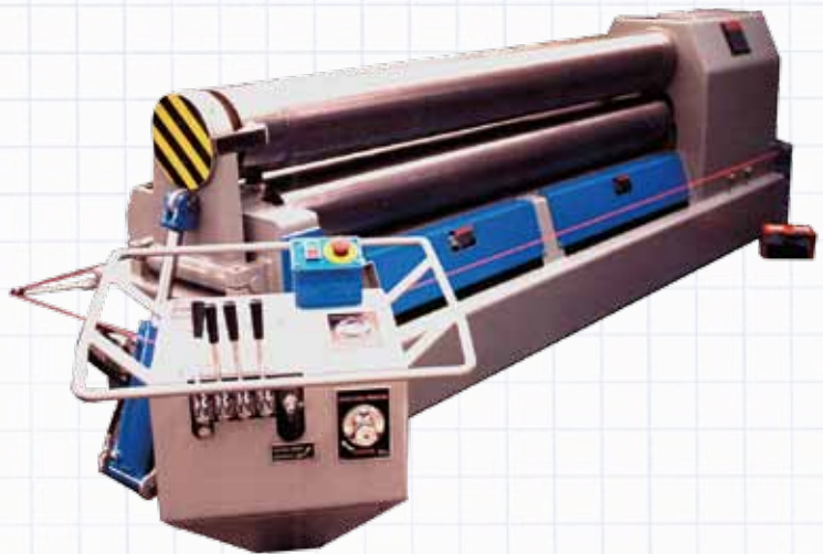
K-10-8 (13/32" x 8') with optional swinging console SC.
