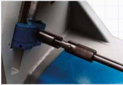
Bending Roll Drive disconnect collar with detent position to allow tilting the back roll for rolling cones and similar parts.
