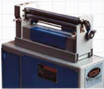
B-1.5-16 power sheet roll (20 gauge x 16") used for filter and silencer manufactures, model makers, labs, and similar applications.
