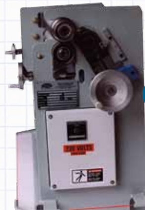
Drop end view of B machine shows location of electrical box, pinch roll adjusting hand wheel, and position scale. Notice the alloy steel bearing case and wedge screw arrangement for accurate positioning of the pinch roll.
