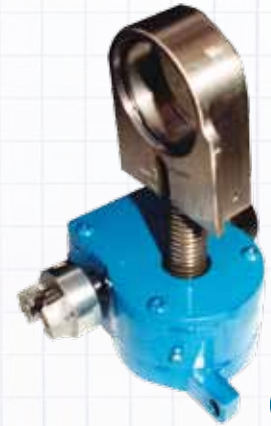
Heavy duty worn gear screw jack arrangement for positioning bending rolls. Alloy steel guide block holds SKF sealed sycpherical roller bearings.
